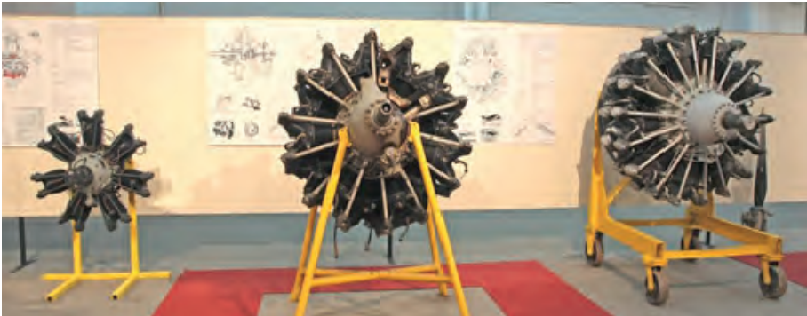
Fig. 9. Radial aero engines, from left to right: Fiat A 50, Fiat A 74, Fiat A 80
