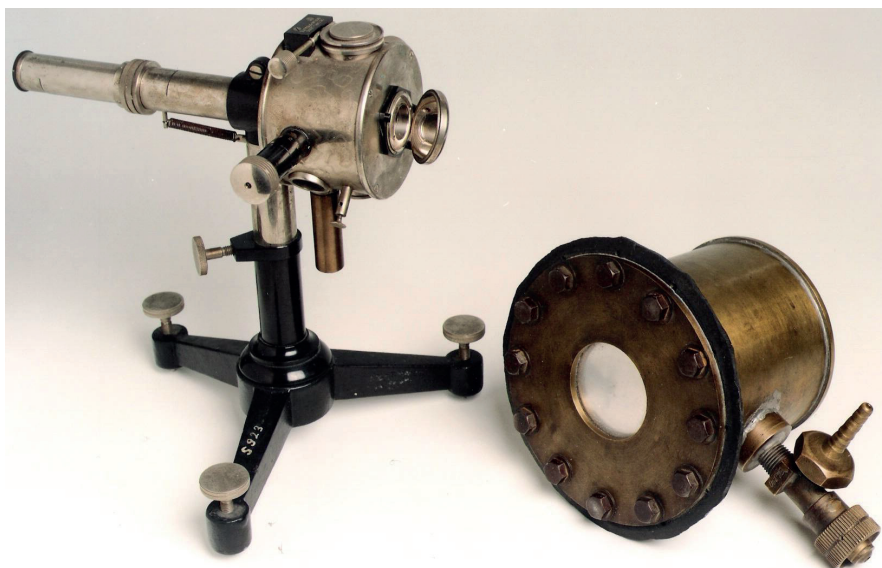
Fig. 1. Ionization chamber and Perucca-type electrometer displayed at the Department of Physics and Chemistry, in the historical building of via Archirafi 36, Palermo (Italy).
